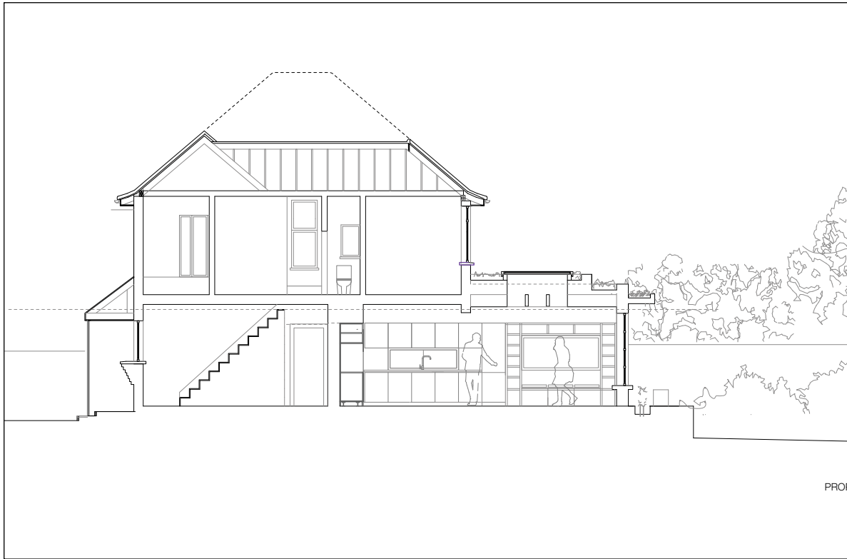
FIGURE 13 Proposed section illustrating a continuation of ground floor levels onto the garden terrace
