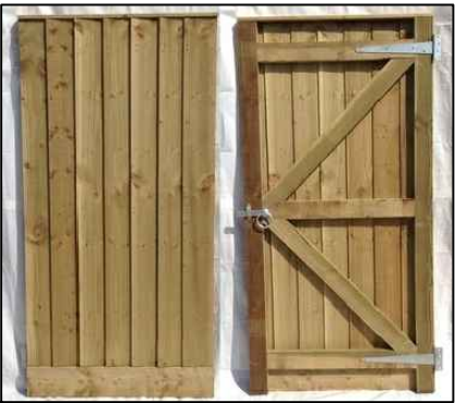
Example of 1.8 Metre high closeboard gate with galvenised hinges, bolt lock and latch/handle attached using stainless steel screws.
