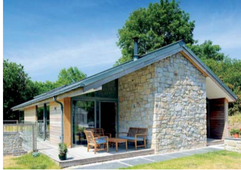
Examples of natural stone, aluminium windows and timber cladding combination
