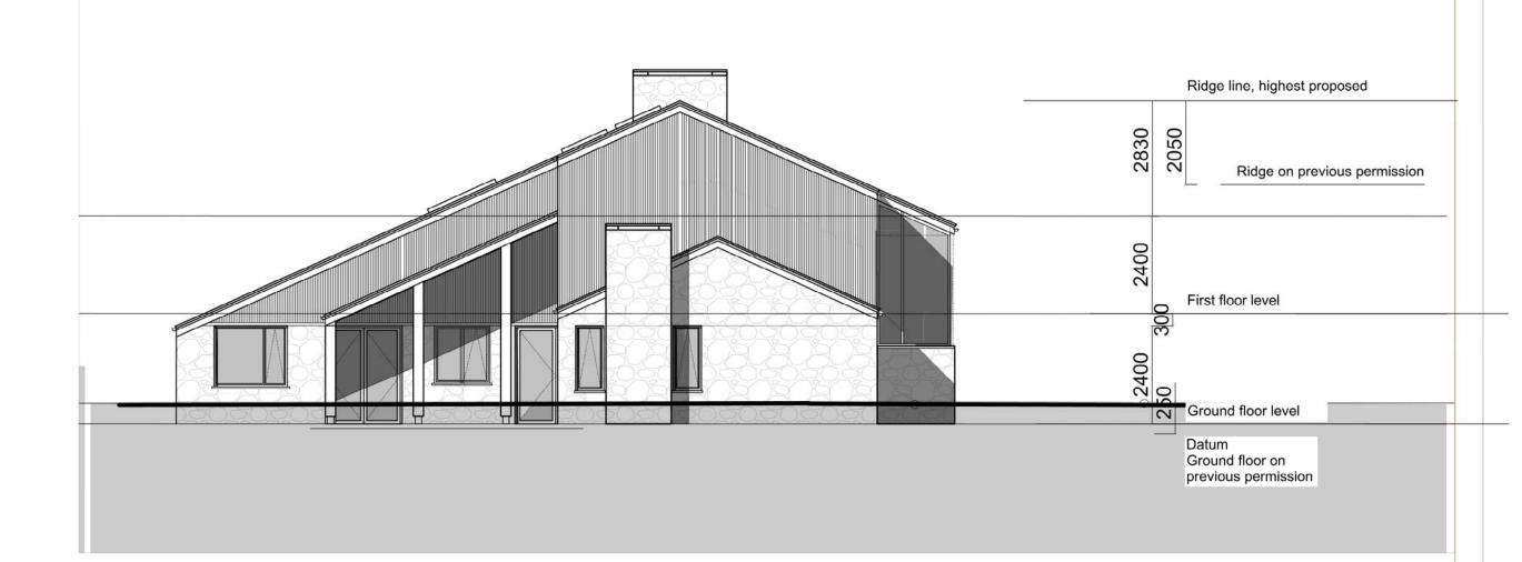
Brynn Mill New House (Enabling Development) West Elevation, As Proposed
