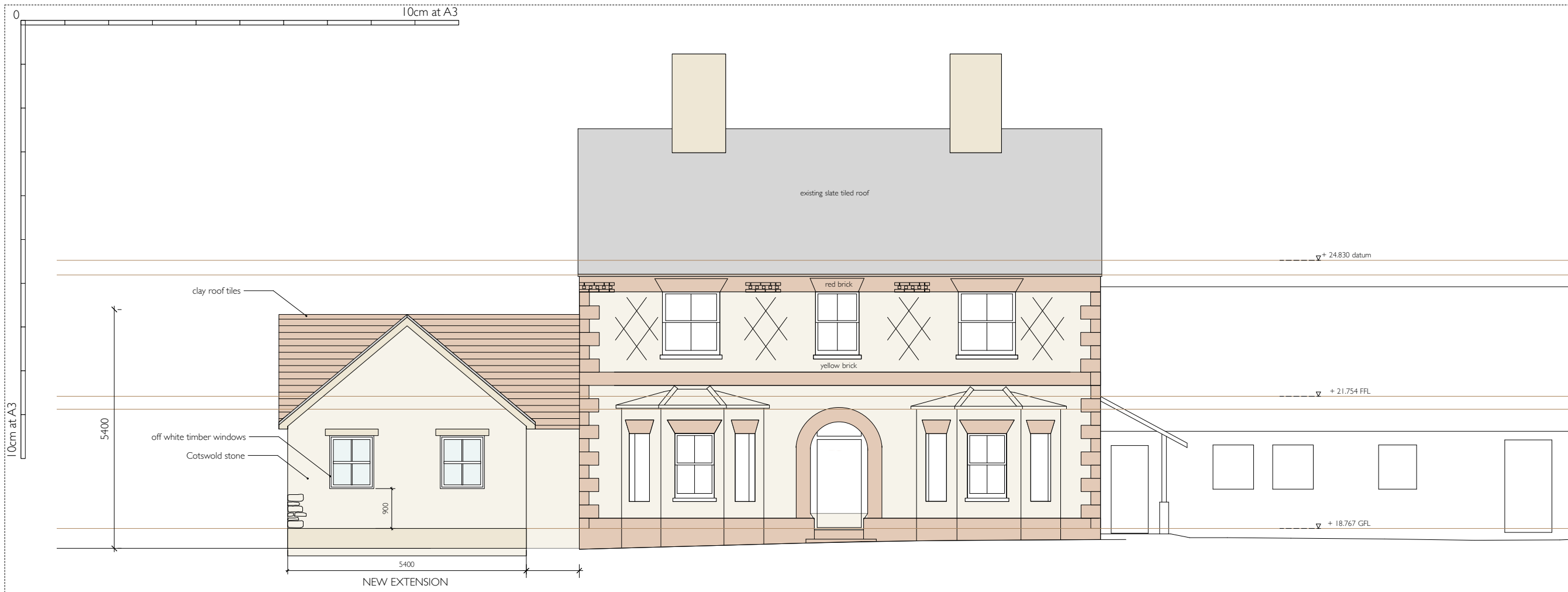
1 Proposed Front (West) Elevation 1:100
