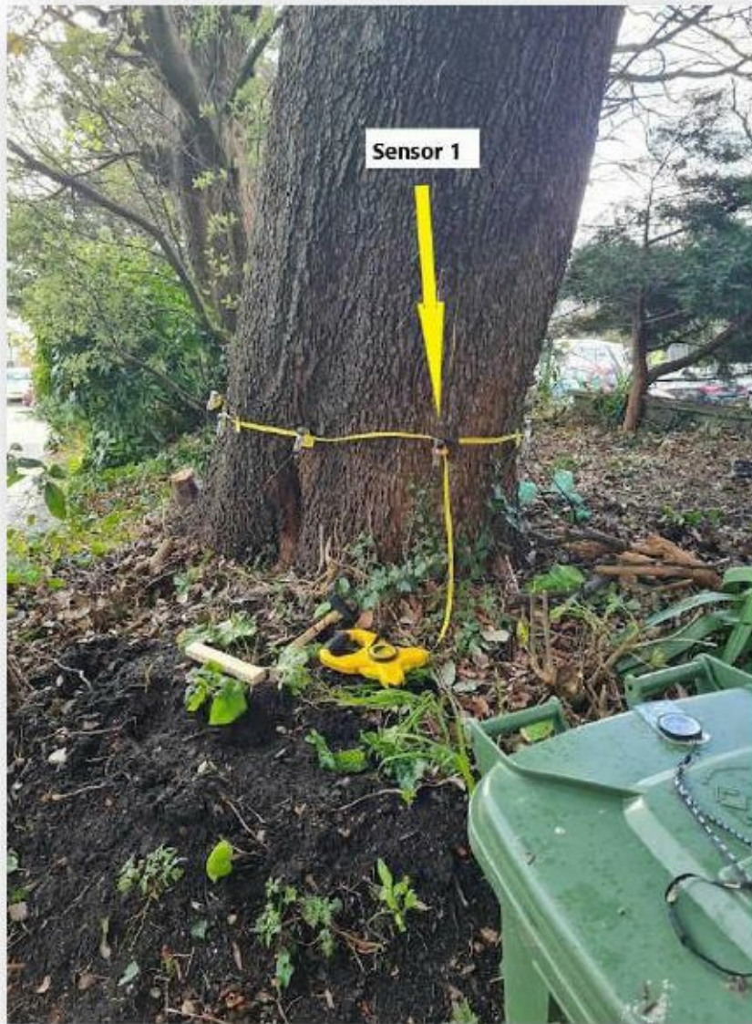
Arborsonic set up looking South (Sensors @ 3500mm)
