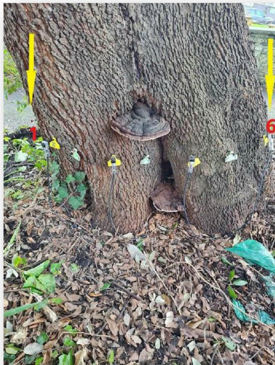
Arborsonic set up between fruiting bodies @ 3500mm- Sensors 1&6 indicated
