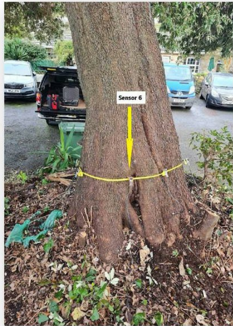
Arborsonic set up looking North (Sensors @ 3500mm)
