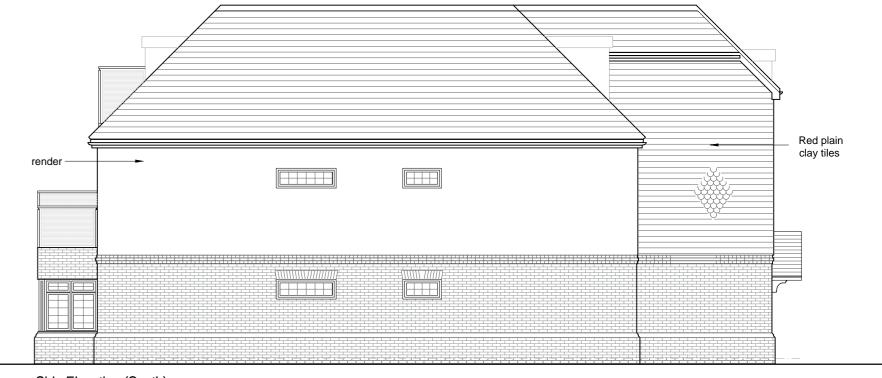
Side Elevation (South) Scale 1:100@A3
