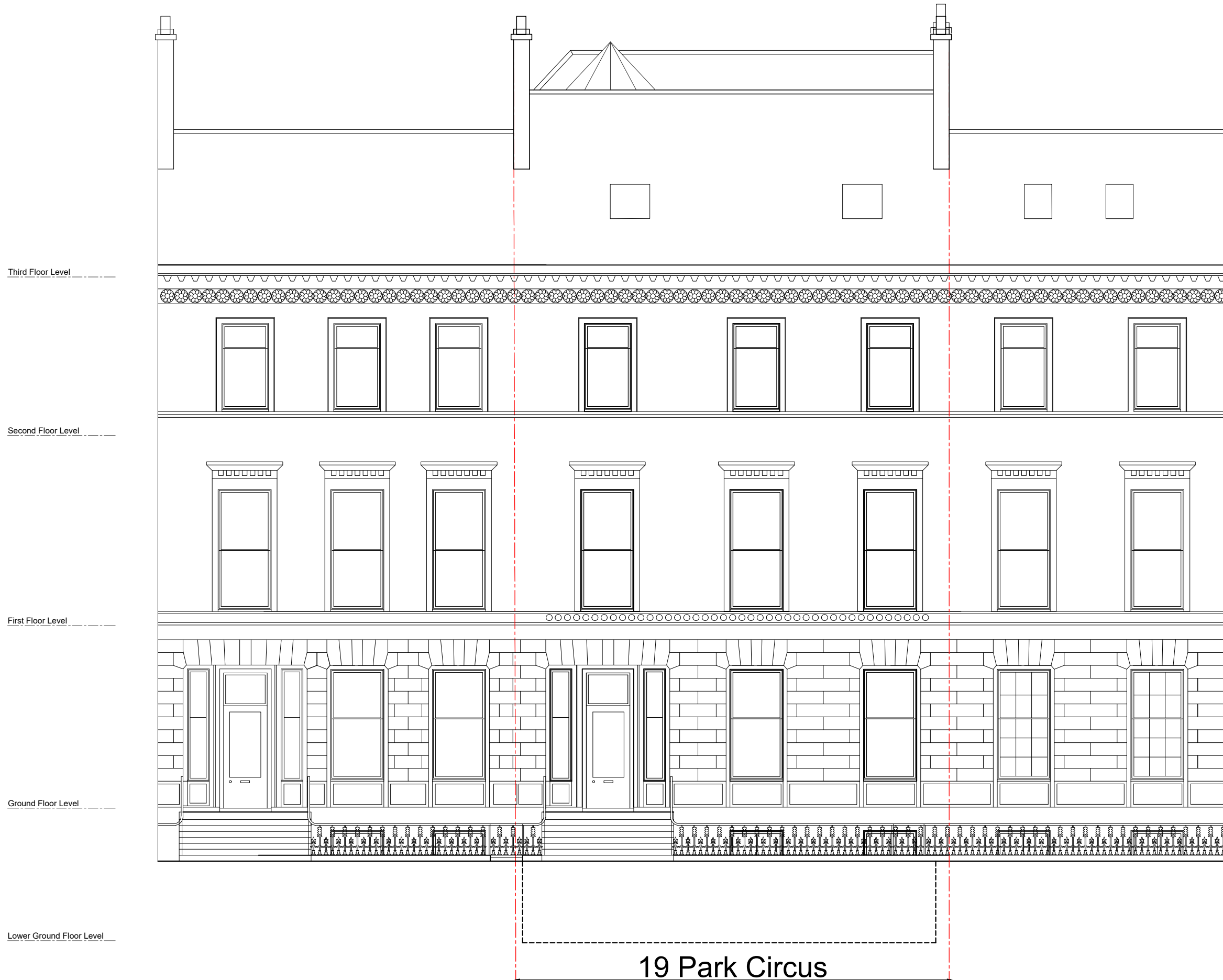
Front Elevation as Existing @ 1:100
