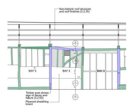
Internal Wall elevation (from Section DD) All wattle and daub infill on this wall in poor condition (3.2.62)
