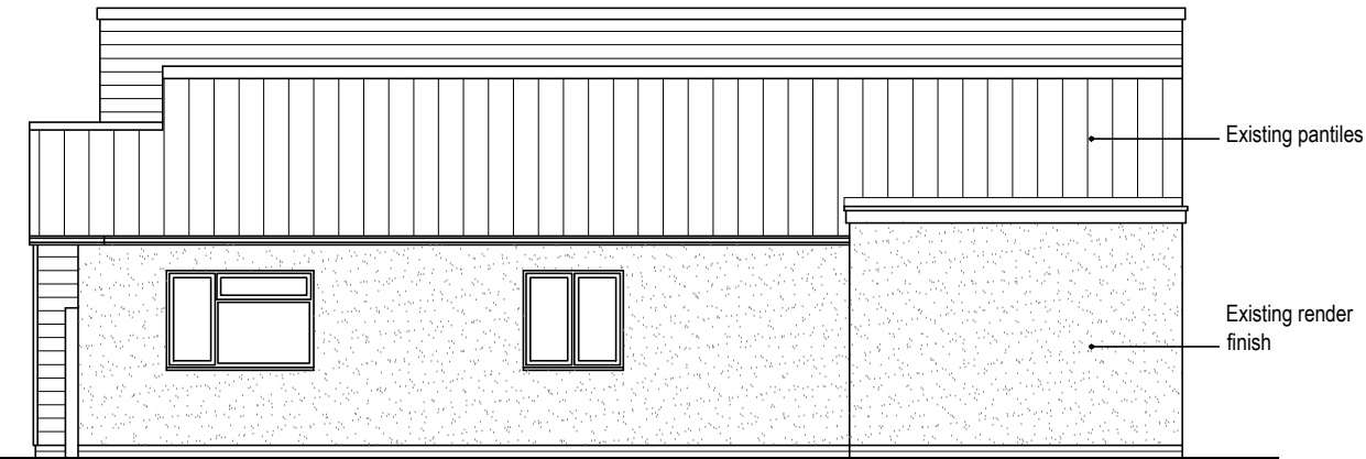
SIDE ELEVATION- existing
