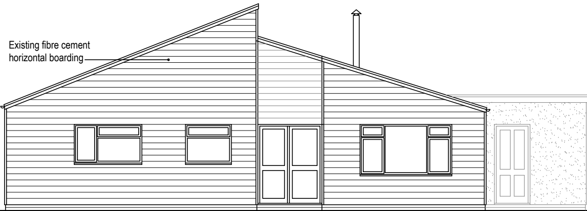
FRONT ELEVATION- existing
