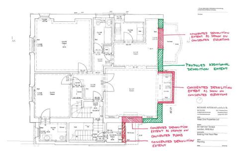
First floor demolition plan - proposed
