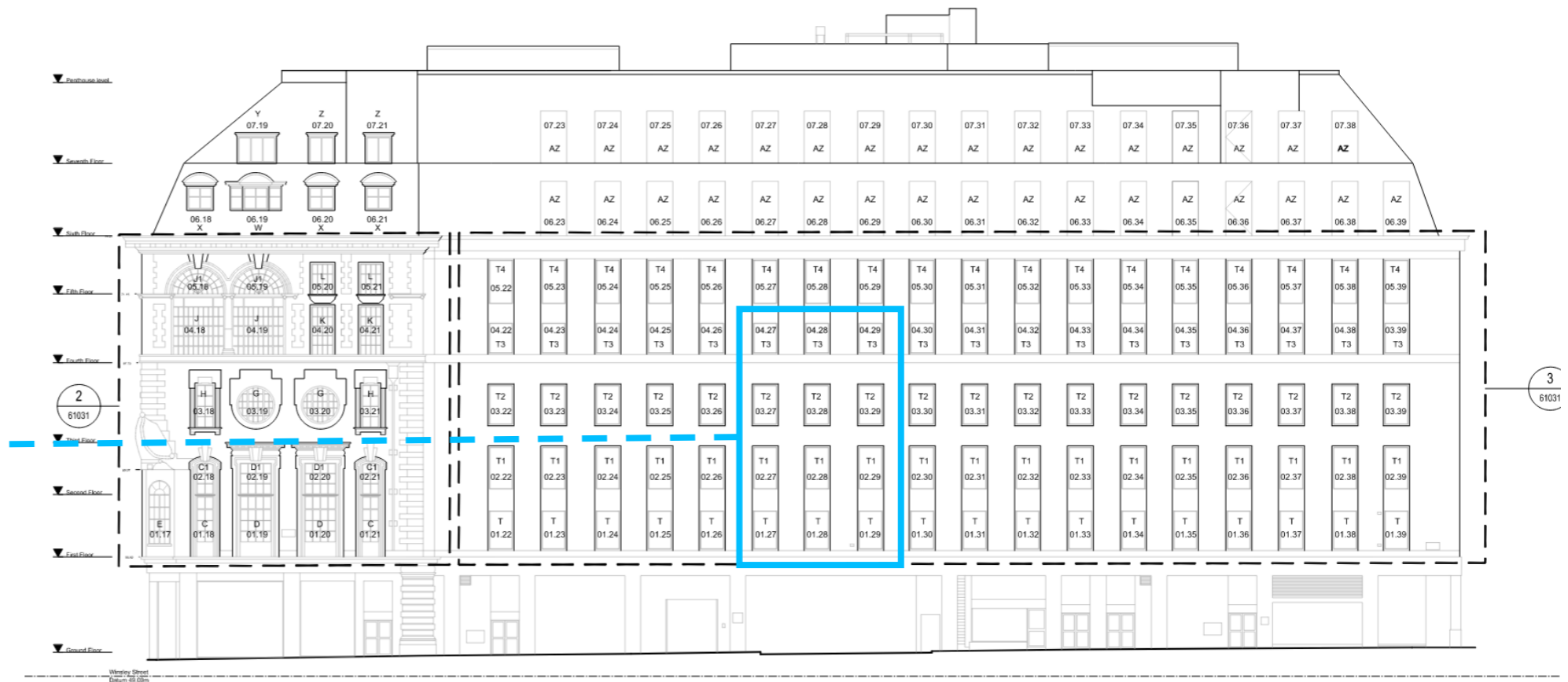
Above: part-elevation of UK House, facing Winsley Street, annotating typical window types
