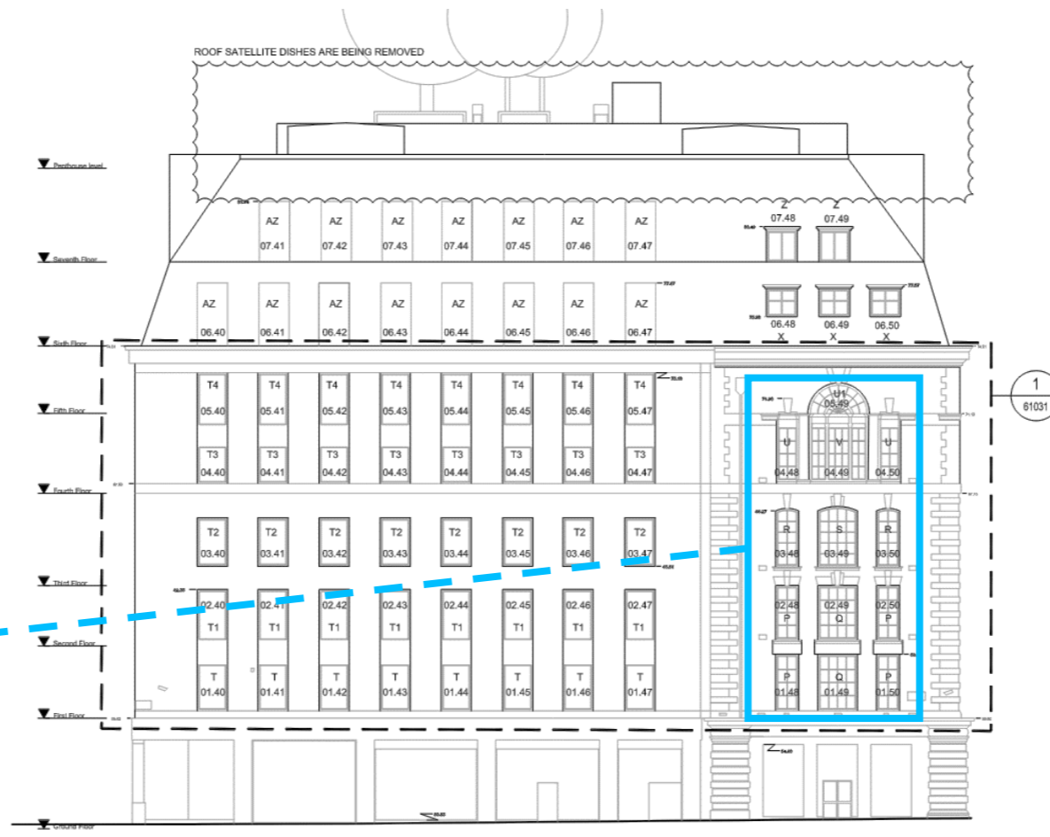
Above: part-elevation of UK in Eastcastle Street, annotating typical timber framed window types
