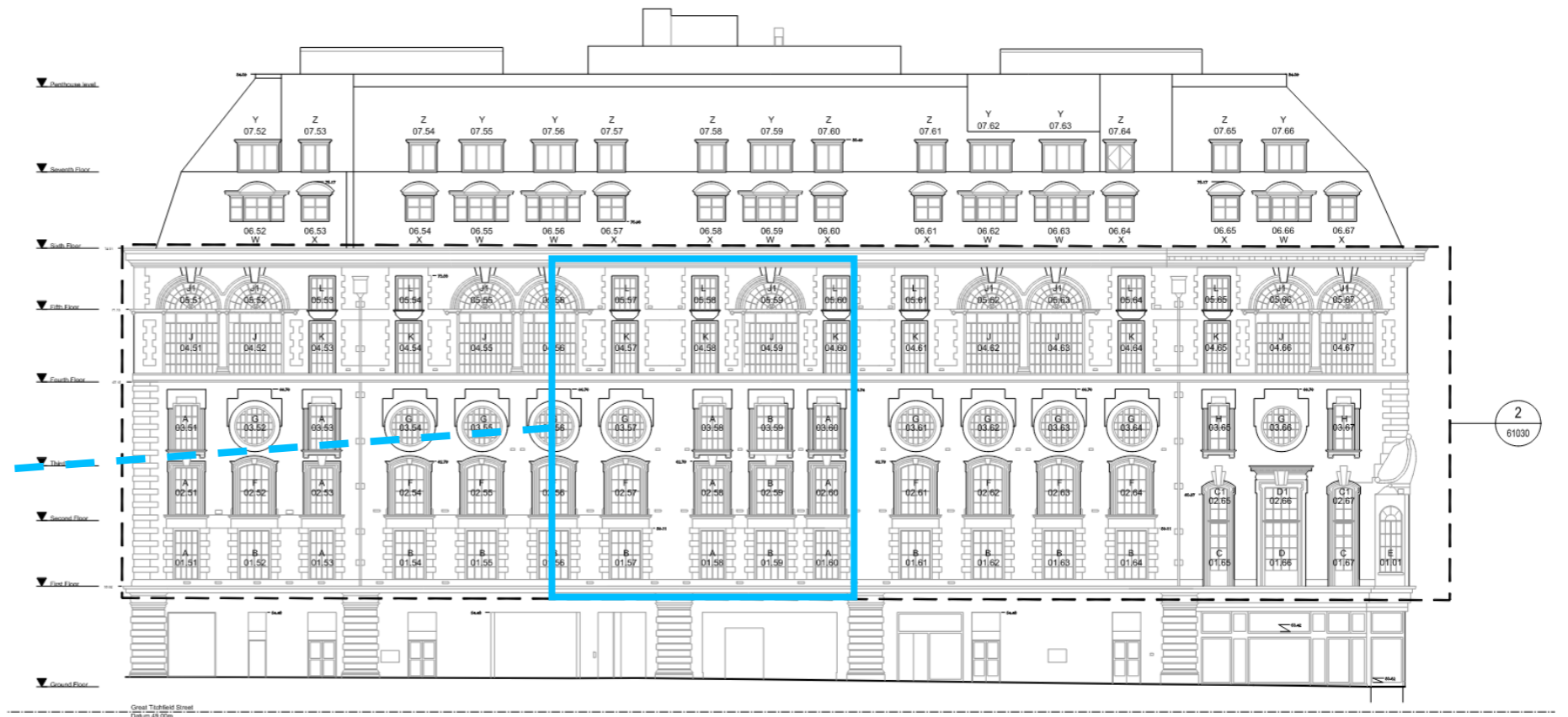
Above: part-elevation of UK in Great Titchfield Street, annotating typical steel window types
