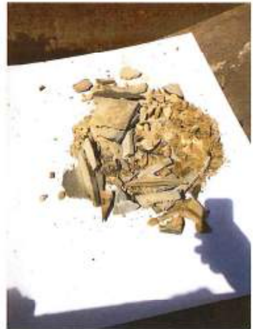
Fig 124: Debris removed during survey 16kg in weight
