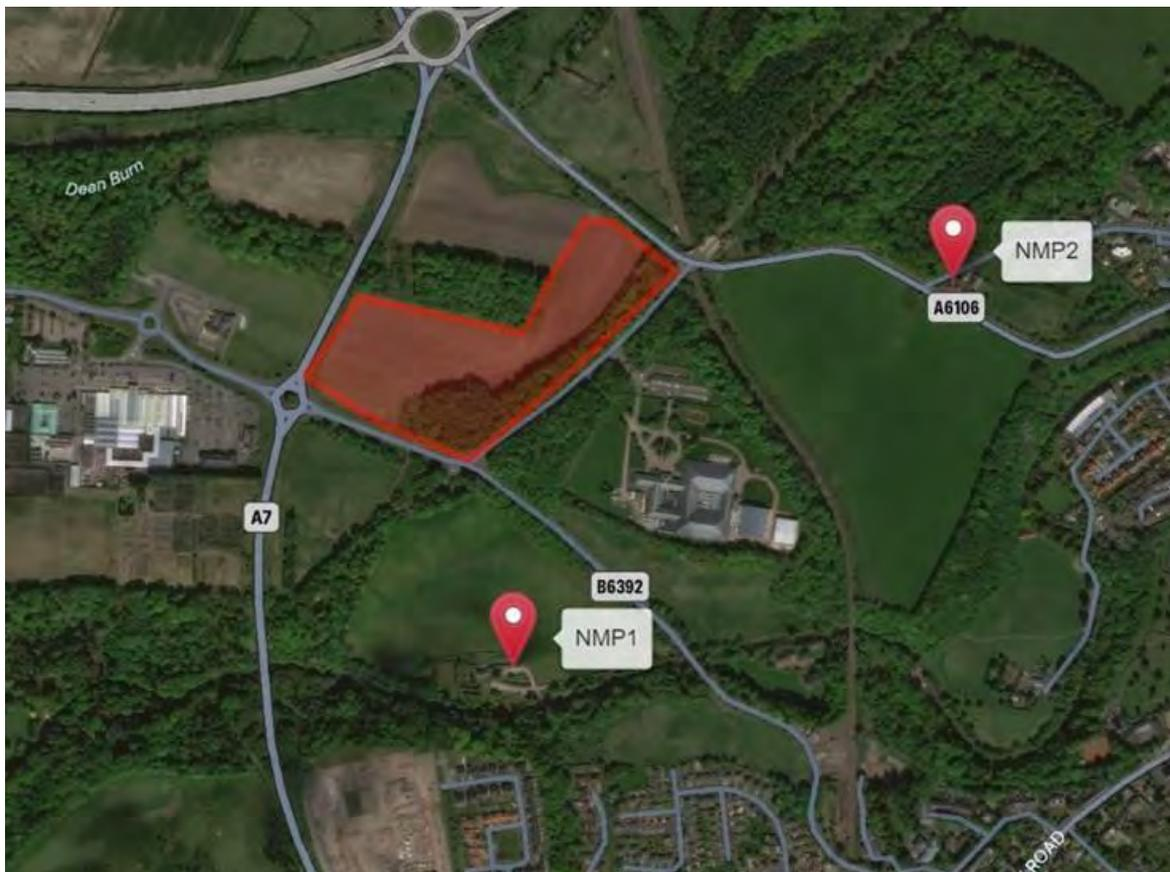
NMP1 – to characterise background noise levels at the existing receptor for evaluation of industrial/commercial noise in accordance with BS4142.
