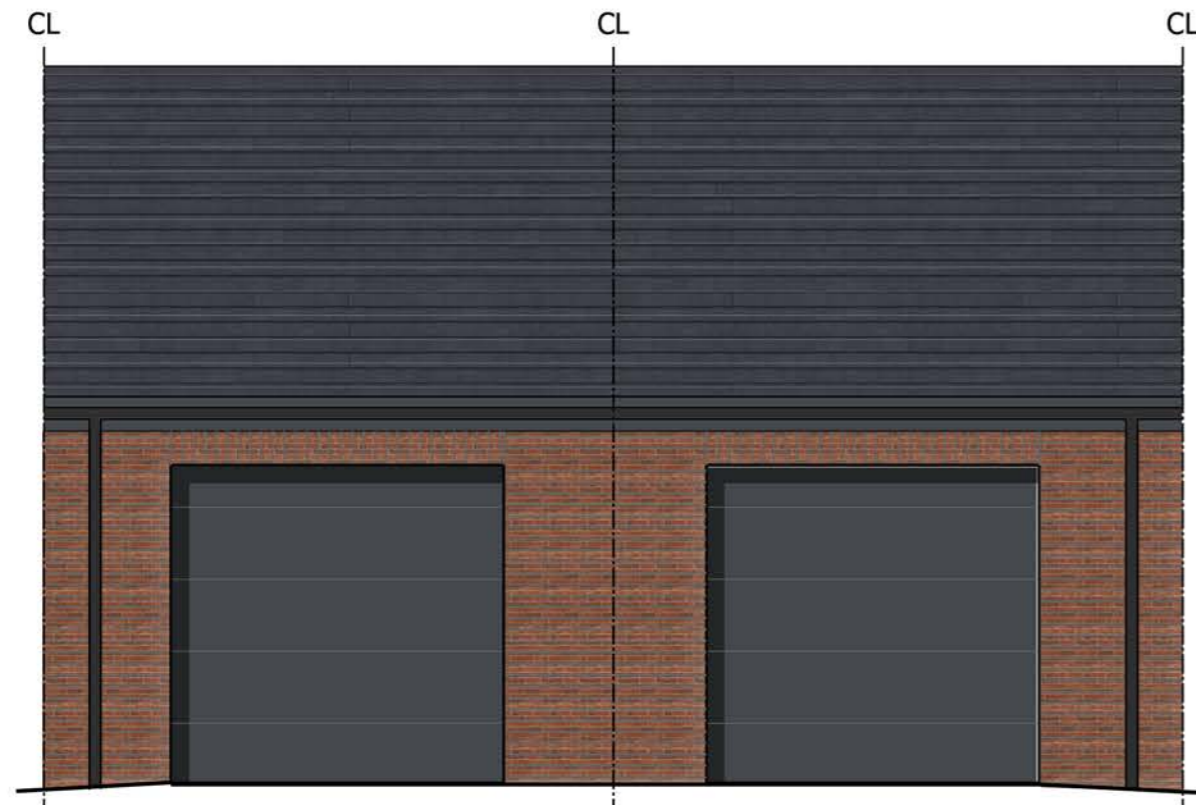
FRONT ELEVATION - SINGLE LINK DETACHED GARAGE
