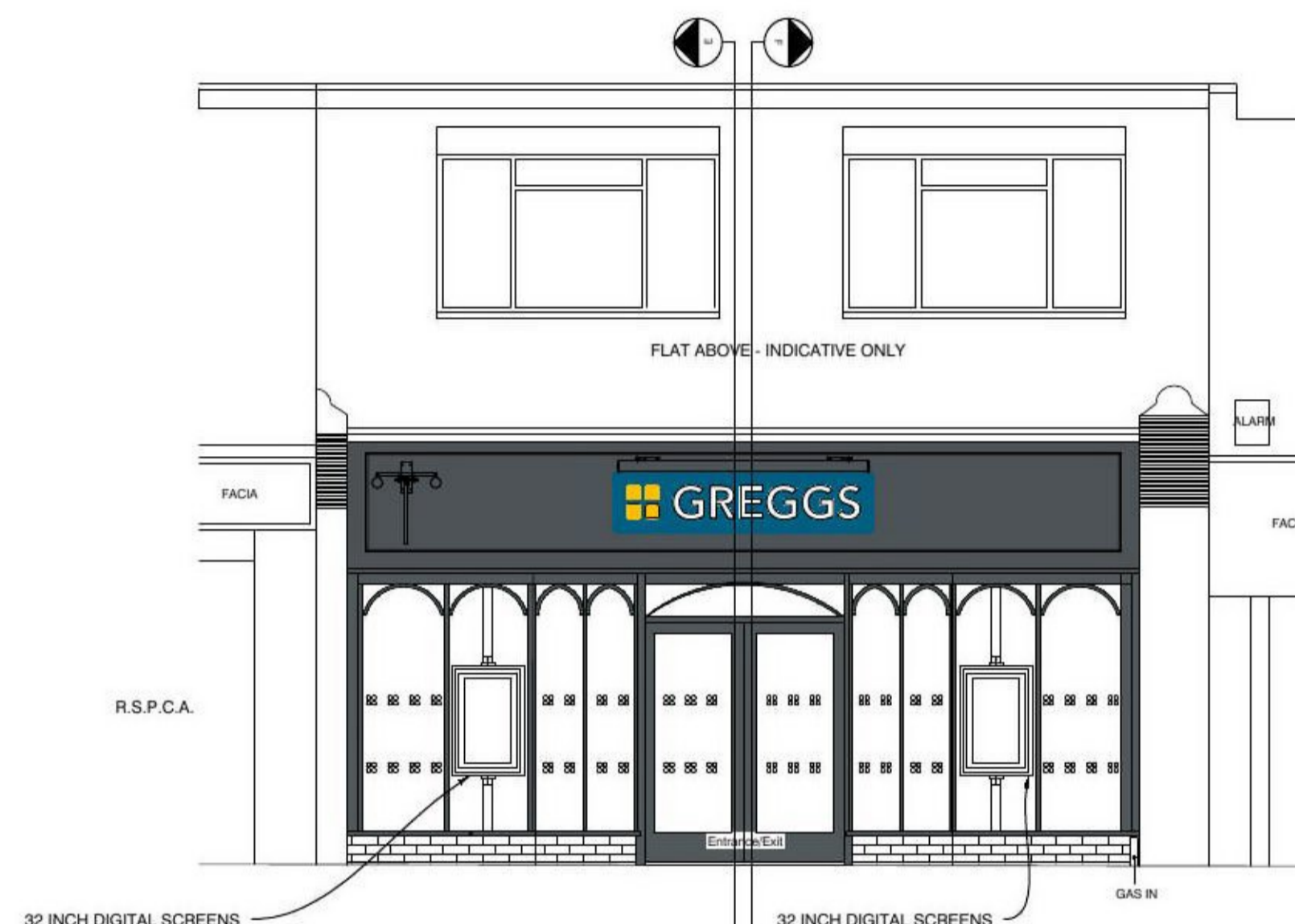
ELEVATION ON PROPOSED SHOPFRONT
