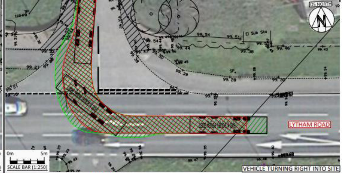
VEHICLE TURNING RIGHT INTO SITE
