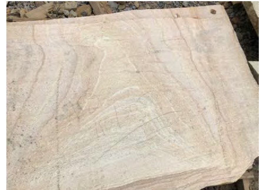
200mm of local stone will be used as the primary facade material across the building, contributing significantly to reducing the embodied carbon of the facades.
