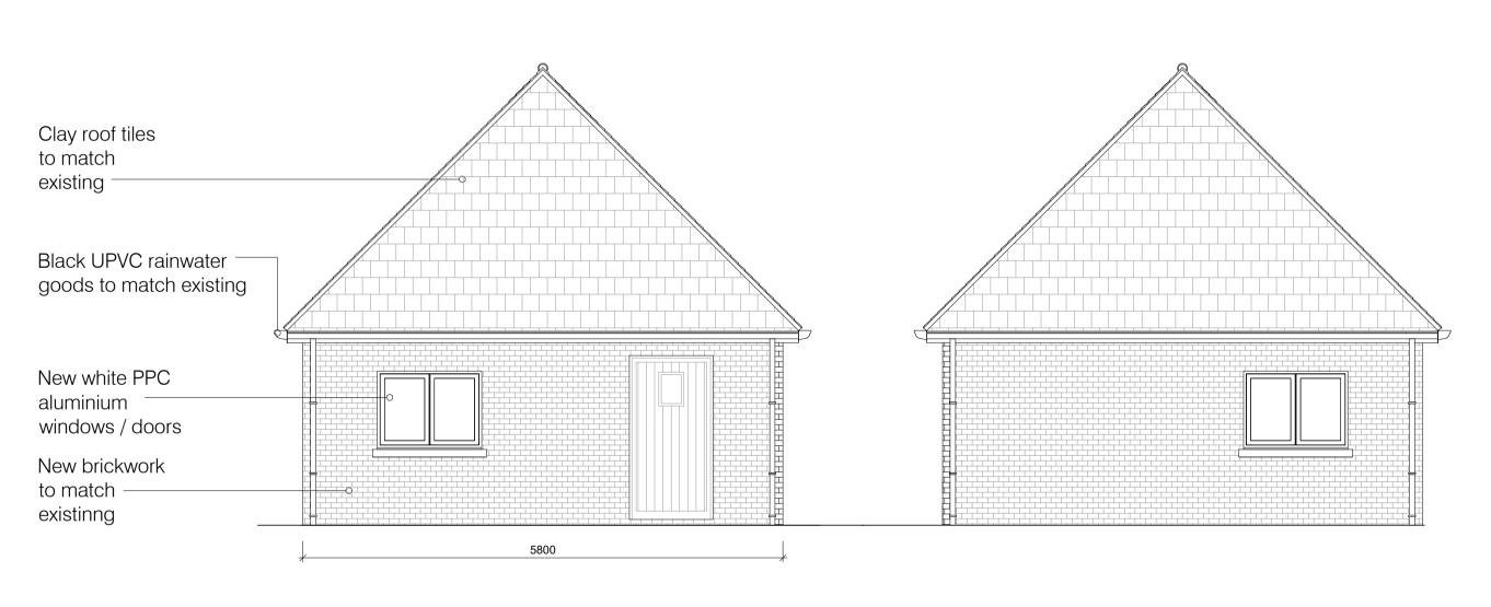
Proposed Right Flank Elevation Proposed Left Flank Elevation
