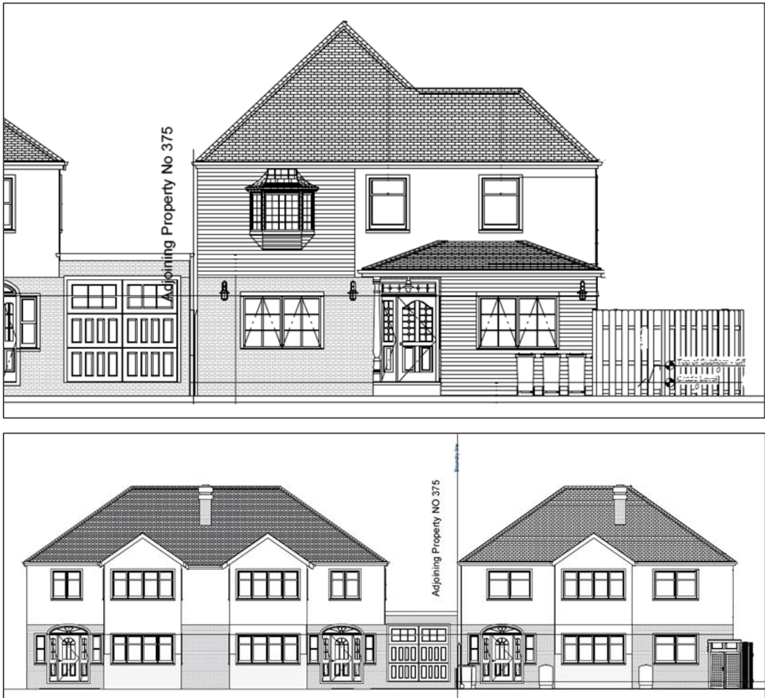
Fig.19: Top image shows front elevation proposed in the pre-application submission and bottom image shows the front elevation now proposed in this application which is shown in context with 375 Malden Road.
