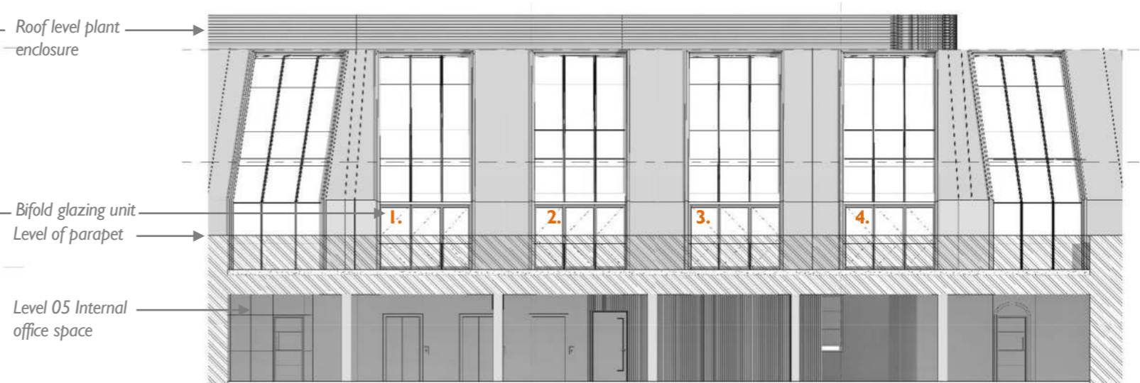
High Level South Sectional Elevation Extract (Parapet in foreground denoted in hatch)
