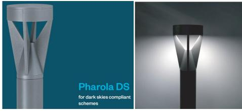
The illumination level using this DS version reduces to less than 0.5 lux at 5.5m from the bollard. It emits zero upward light.
