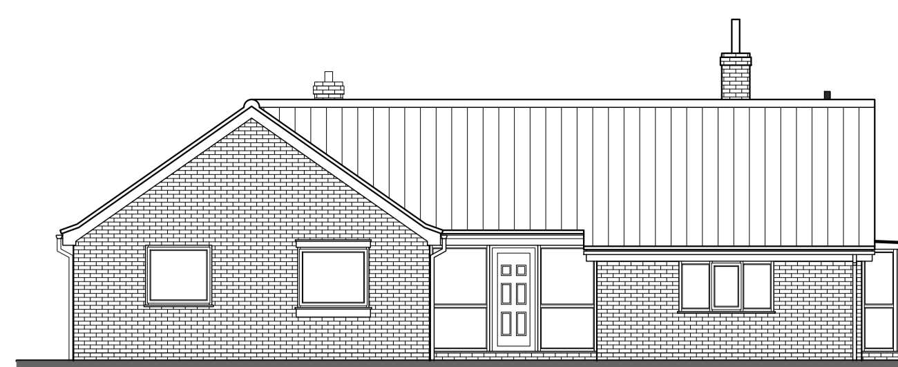
PROPOSED FRONT ELEVATION SCALE: 1:100
