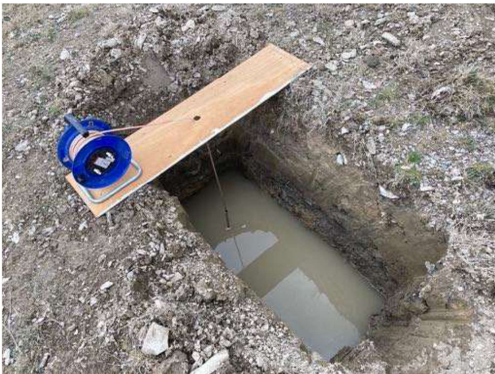
Photograph 14 Description: Water level monitoring at trial pit TP01 (end of test) Date: 28/04/2021 Location: North western part of Site A
