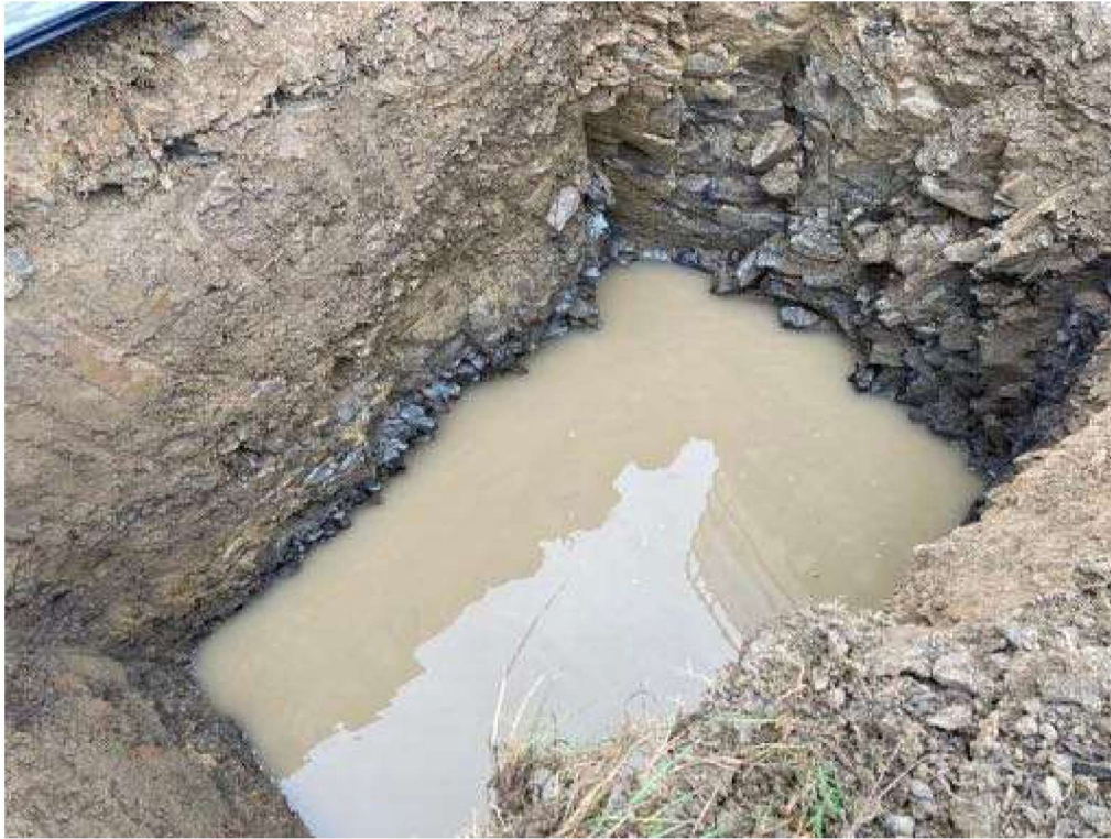
Photograph 17 Description: Inundation of trial pit TP02 (start of test) Date: 28/04/2021 Location: North western part of Site A
