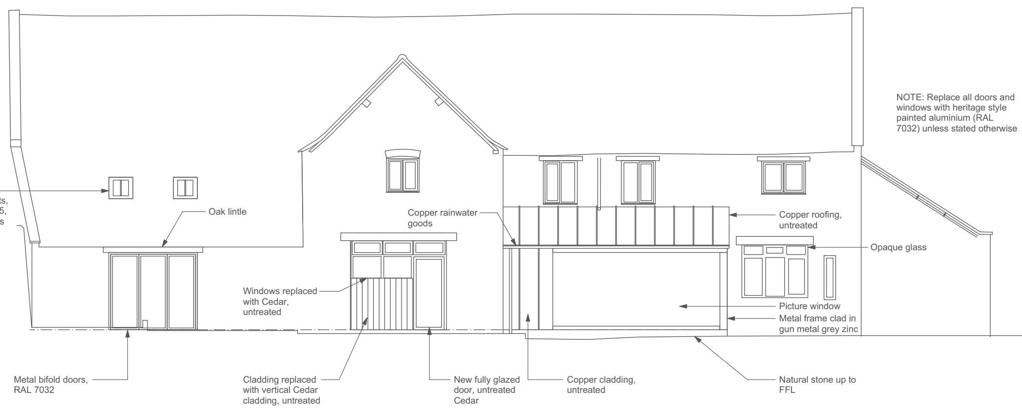
NORTH WEST ELEVATION
