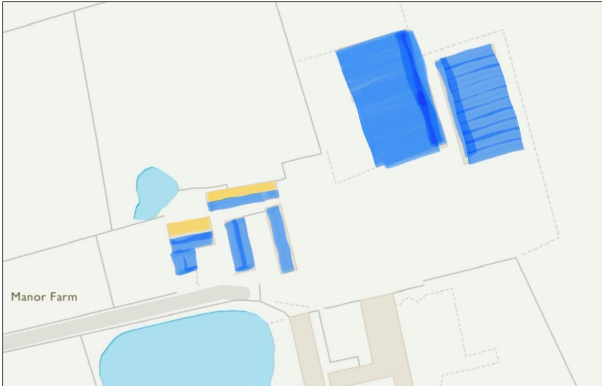
Figure 25 The buildings in blue drain into the large pond and yellow into the small pond to the north
