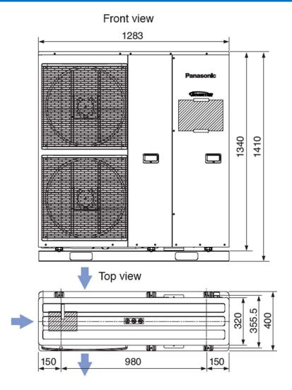
Dimensions of compact unit with two fans in mm. The air flow is depicted by arrows.
