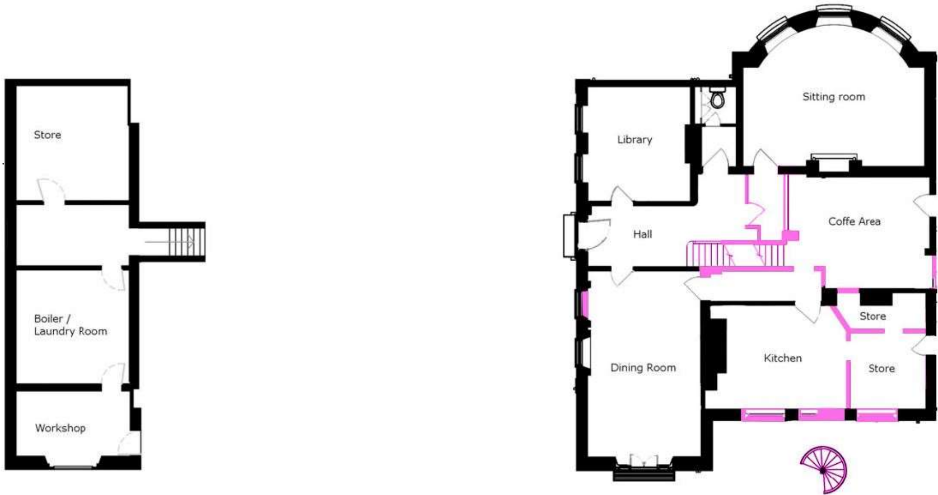
Figure 58: Proposed Demolition Plan – Basement and Ground Floor
