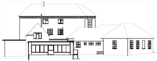
Existing rear elevation (west elevation) with current 20 th Century extensions proposed for removal
