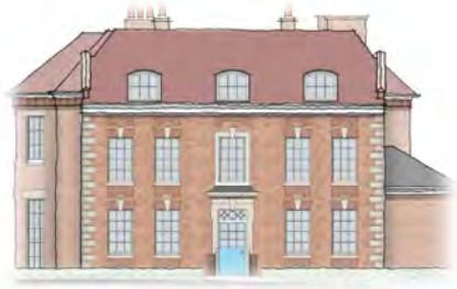
Proposed principal elevation – showing removal of 20 th Century extensions and new dormer windows.
