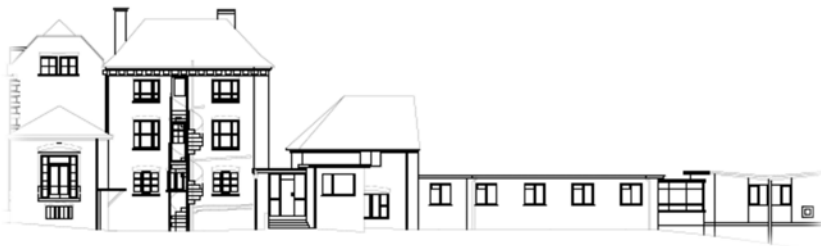
Existing side elevation (North Elevation) with external spiral commercial stair case and sprawling 1960s and 1980s extensions
