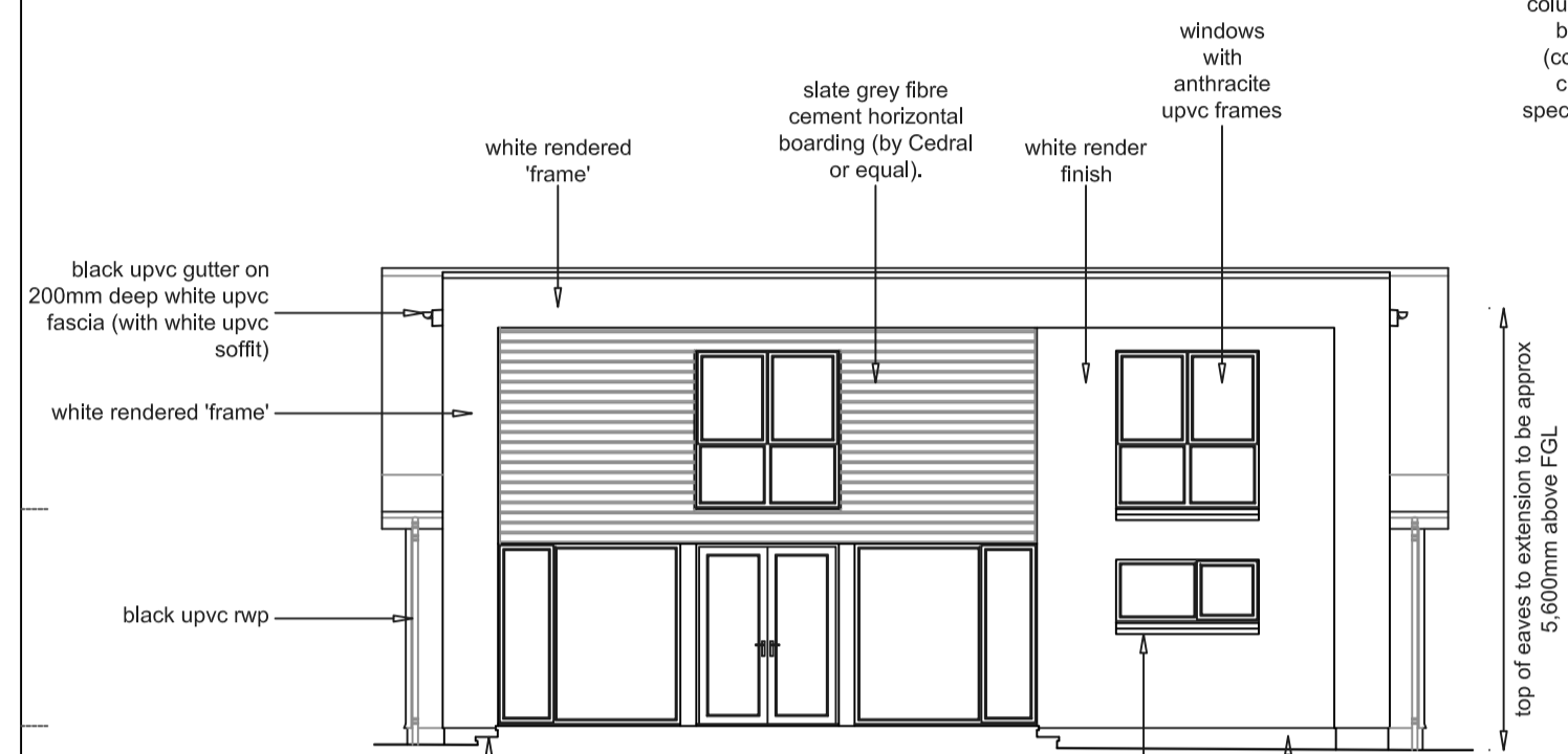
HOUSE:- Rear (South) Elevation
