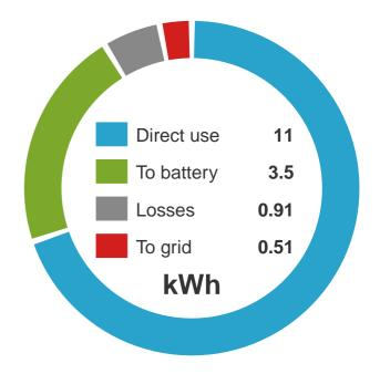
This graph shows the modelled profile of electricity generated by the PV array on a selected day (March 27th). On this day the PV system is expected to generate 16.3 kWh. Of this, 11.4 kWh (70%) is used directly in the property, 4.4 kWh (27%) is stored in the battery for later re-use, and 0.5 kWh (3%) is exported to the grid.
