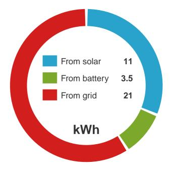
This graph shows modelled consumption data over the course of the selected day (March 27th). Total electricity consumption on this day was 37.3 kWh, of which 11.4 kWh (31%) is expected to be supplied directly by the solar array, and a further 3.5 kWh (9%) drawn from the battery storage system. The remaining 21.5 kWh (58%) is imported from the grid.
