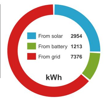
The property is expected to consume 11500kWh of electricity each year. Around 26% of this (2954 kWh) is expected to be supplied directly by the solar array. Another 11% (1213 kWh) is supplied from the storage battery. The remaining 64% (7376 kWh) is supplied from the grid.
