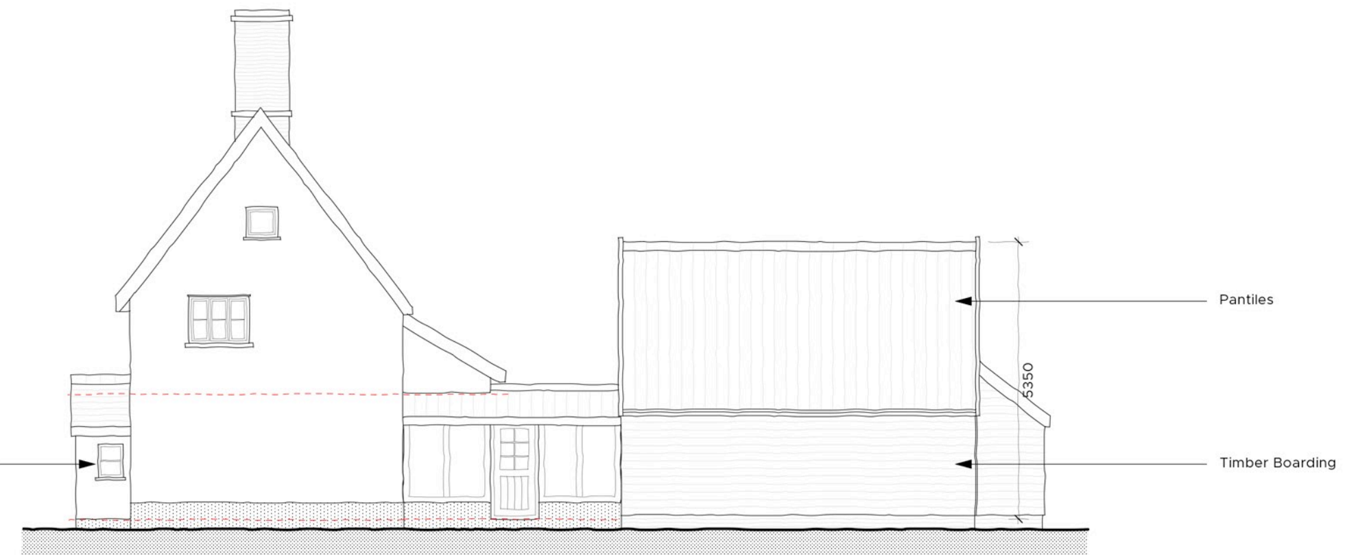
EXISTING EAST ELEVATION (SIDE)
