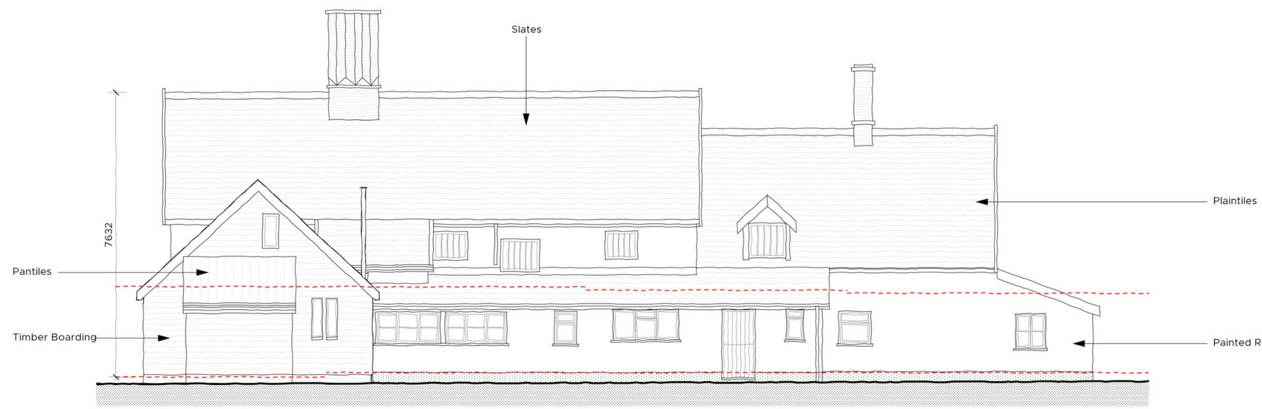
EXISTING NORTH ELEVATION (REAR)
