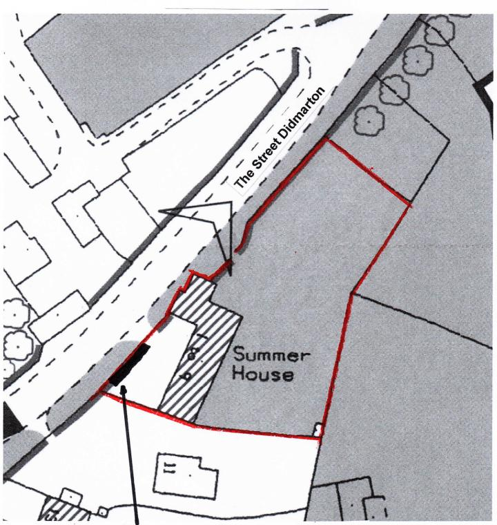
ERECTION OF REPLACEMENT WALL 8m long 2.3m high .5m width To match adjacent wall Stone recovered from wall when it fell down Same colour sand and cement mix
