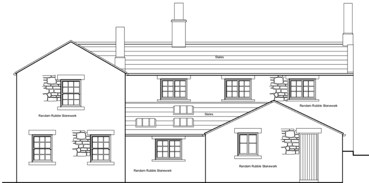
North elevation as existing
