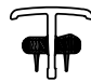
Shaded portions of 2mm Coupler removed where shown, to avoid internal ribs of Cill
