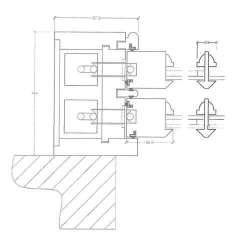
Sash window horizontal cross section 6 Ponsonby Place Scale 1:2
