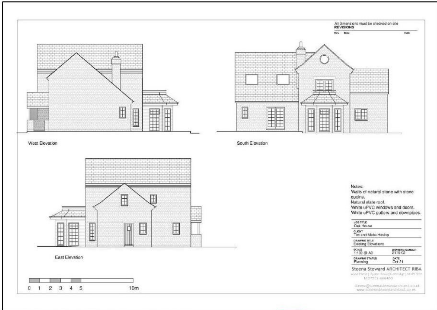
Figure 2. Existing elevations of main dwelling.
