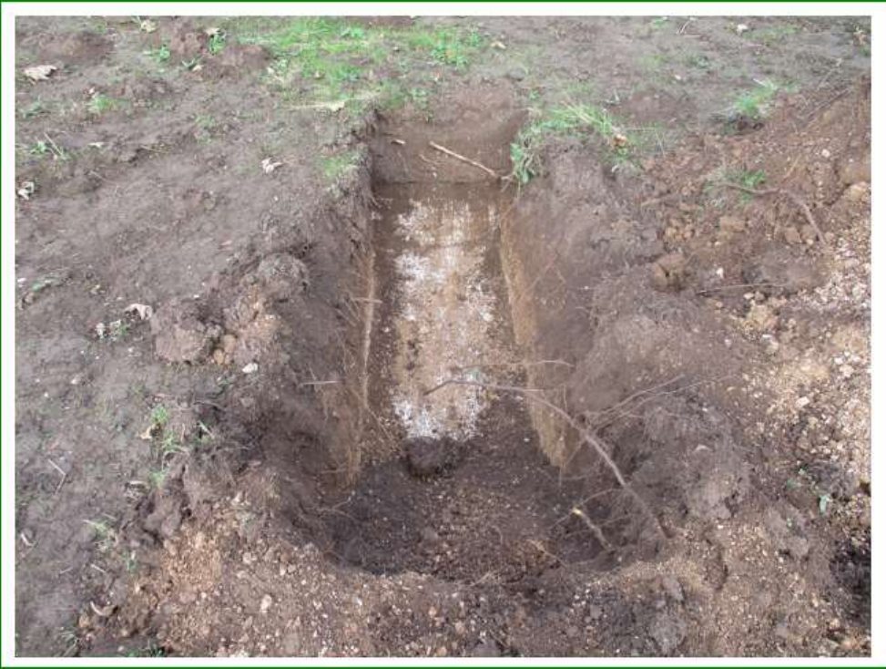
Photo No.14: One of 2 No. small pits noted in the NE and NW corner of sites showing topsoil atop residual bedrock chalk
