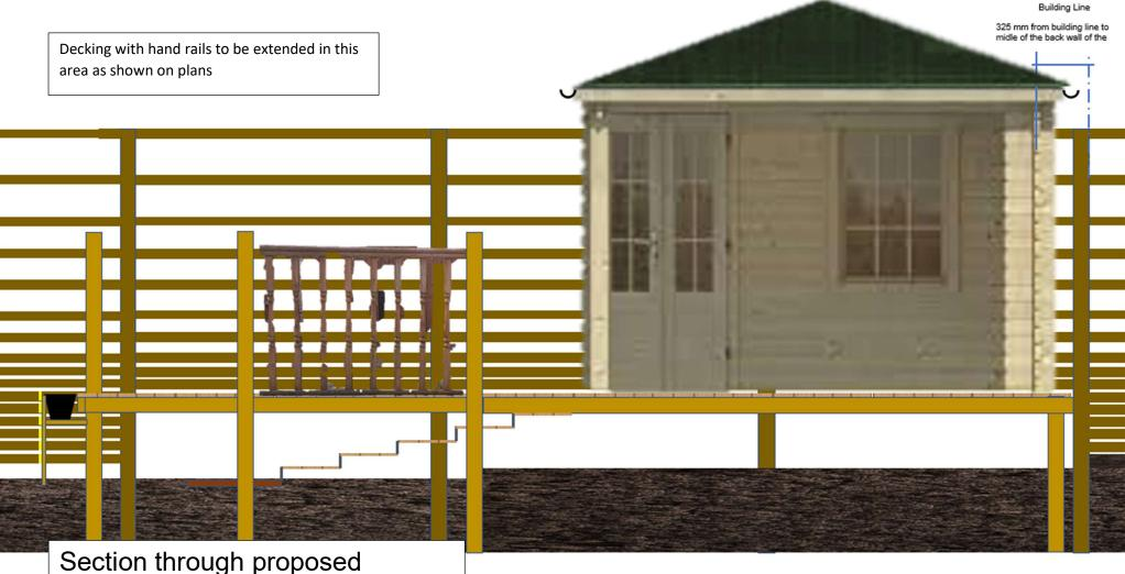
Section through proposed Summerhouse and decking at A-A
