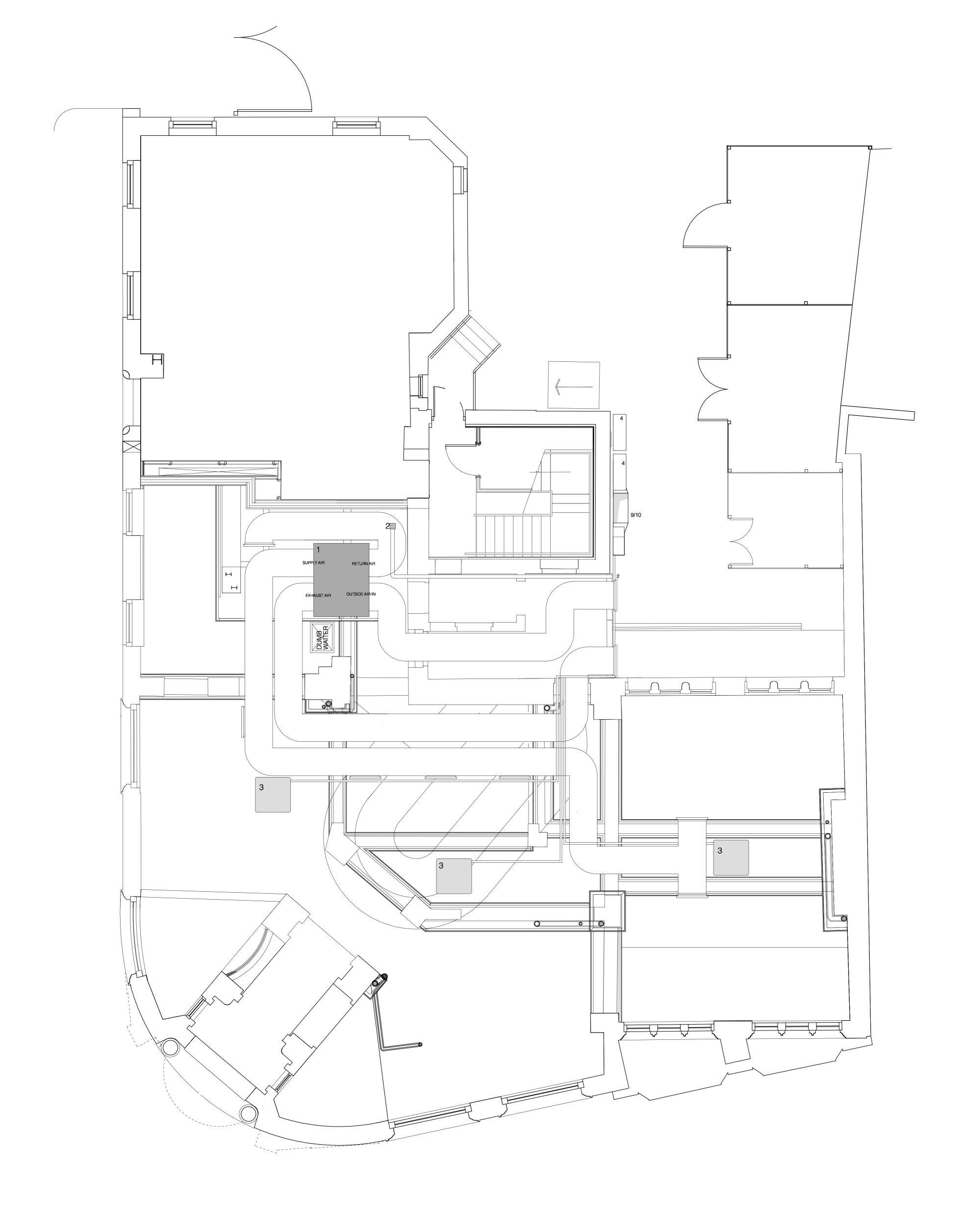
1. MITSUBISHI LGH 250 RVXT-E, LOSSNAY HEAT RECOVERY UNIT MOUNTED AT HIGH LEVEL ABOVE DISABLED TOILET. 750X250MM DUCTWORK TO FOLLOW ROUTES SHOWN TIGHT TO CEILING LEVEL. DUCTS TO EXTERIOR TO RUN AT HIGH LEVEL ACROSS STAIRCASE AND ABOVE WINDOW OPENING TO TERMINATE ABOVE EXIT DOOR AND LIGHTWELL WALL WHICH IS A NON ORIGINAL PART OF THE BUILDING FABRIC.
