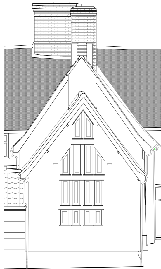
Existing East Elevation Window Arrangement
