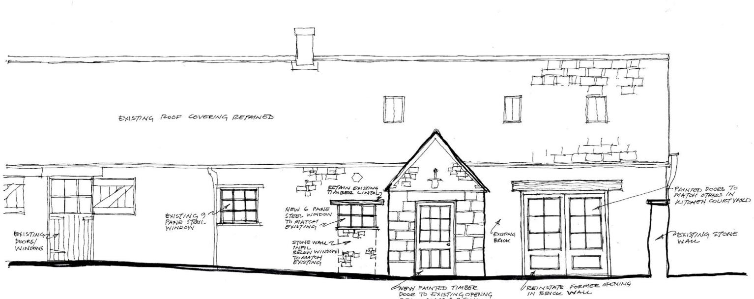
NEW PAINTED TIMBER Door TO EXISTING OPENNG 9 PANE GLASS & & SOLID PANELS TO BASE
