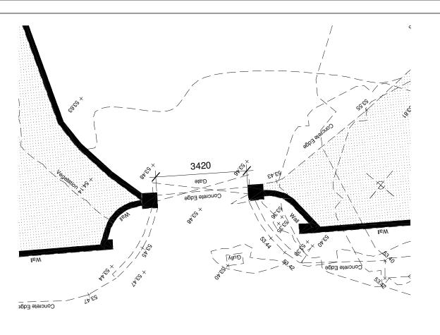
Existing brick posts to be \_taken down and rebuilt to create wider opening to allow easier access.
