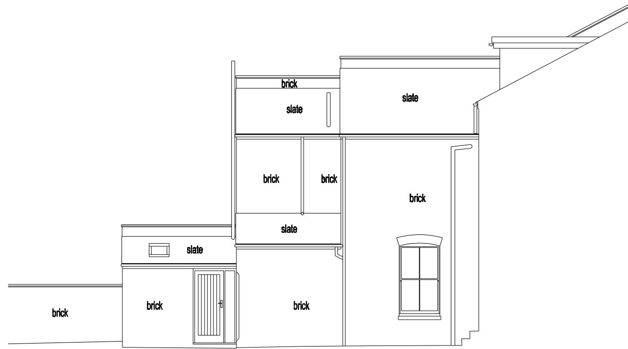
SIDE ELEVATION Southeast
