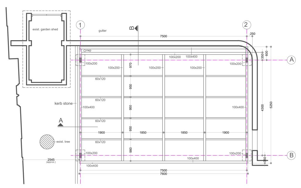
Plan - Glulam Wood Roof Construction
