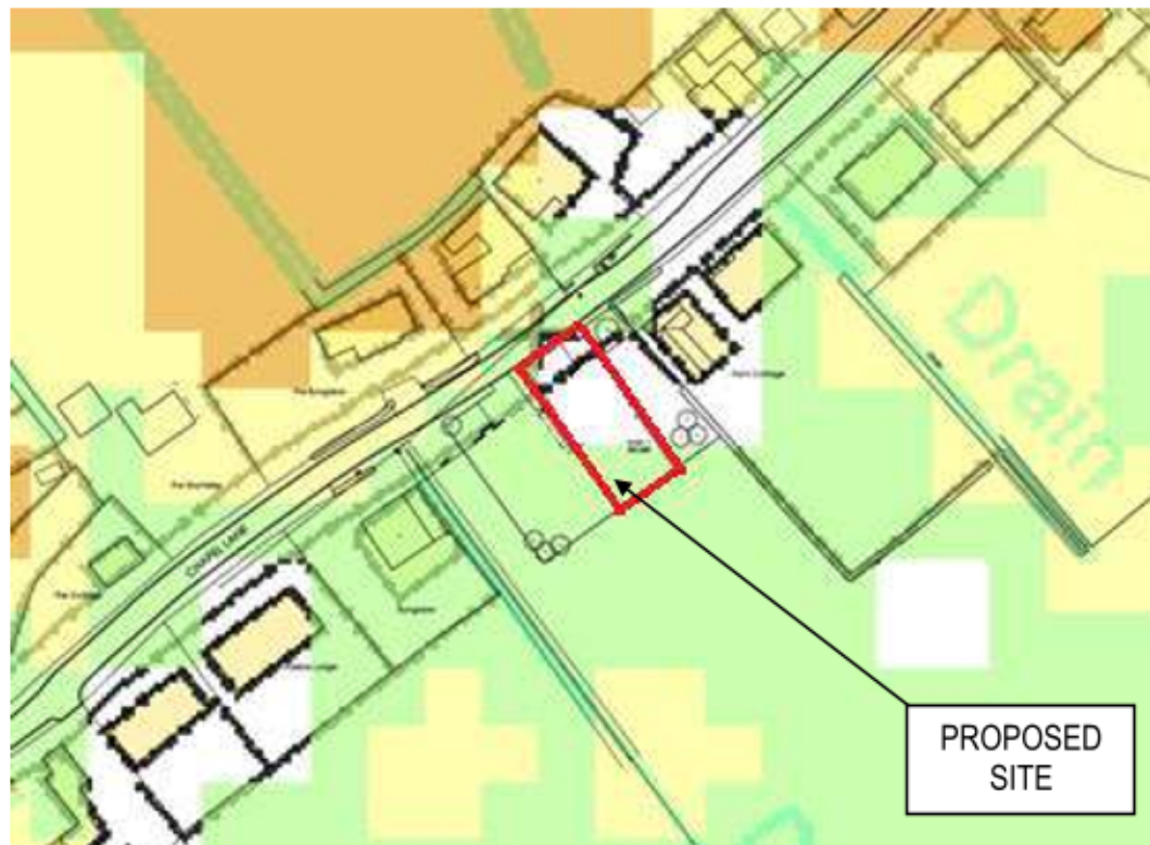
FIGURE 7: Hazard rating map for a 1 in 200 year breach (scenario year 2115) with red line boundary
