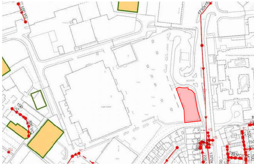
Figure 2.0 Existing Drainage – United Utilities Records
