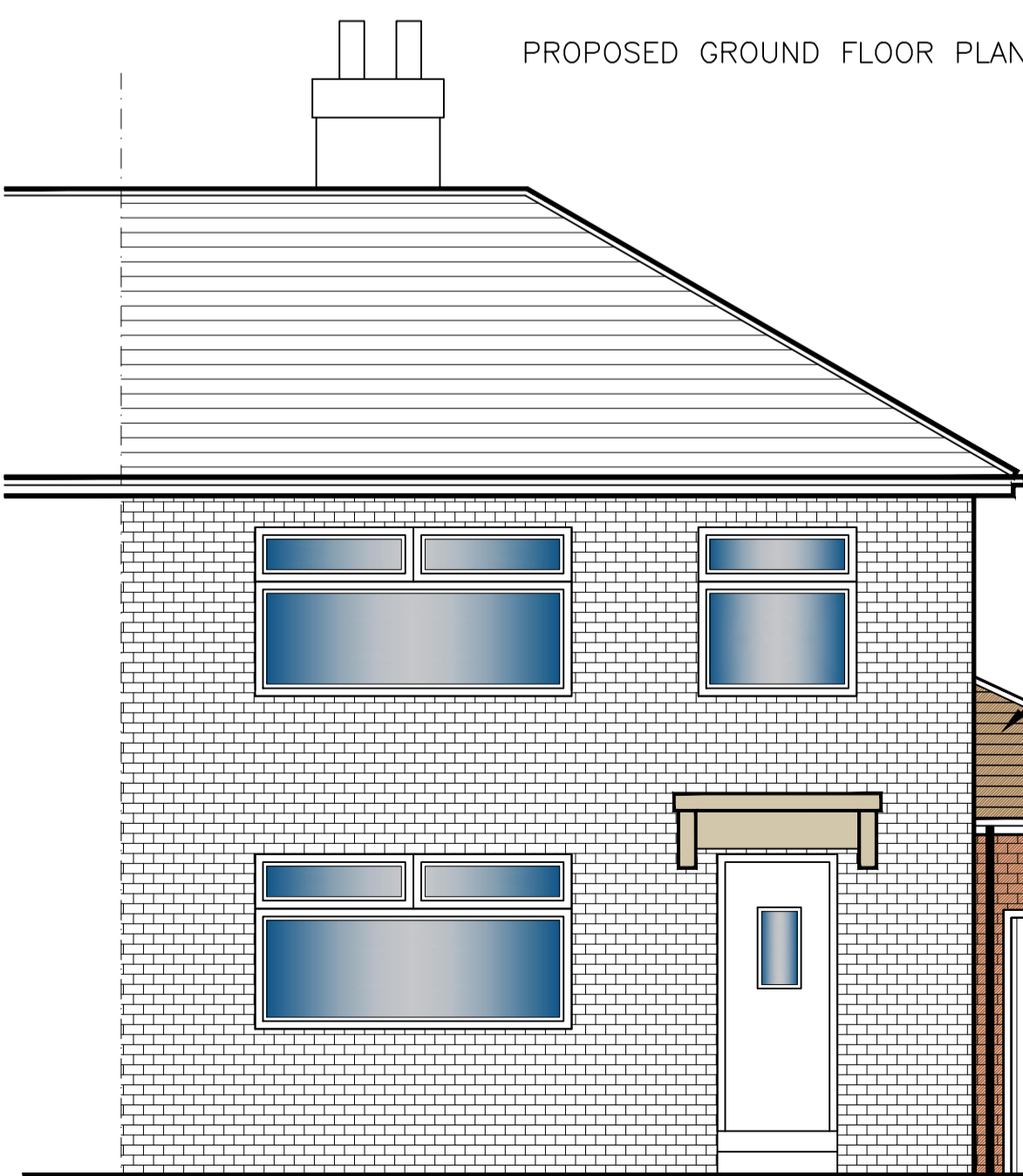
PROPOSED FRONT ELEVATION (1:50)
