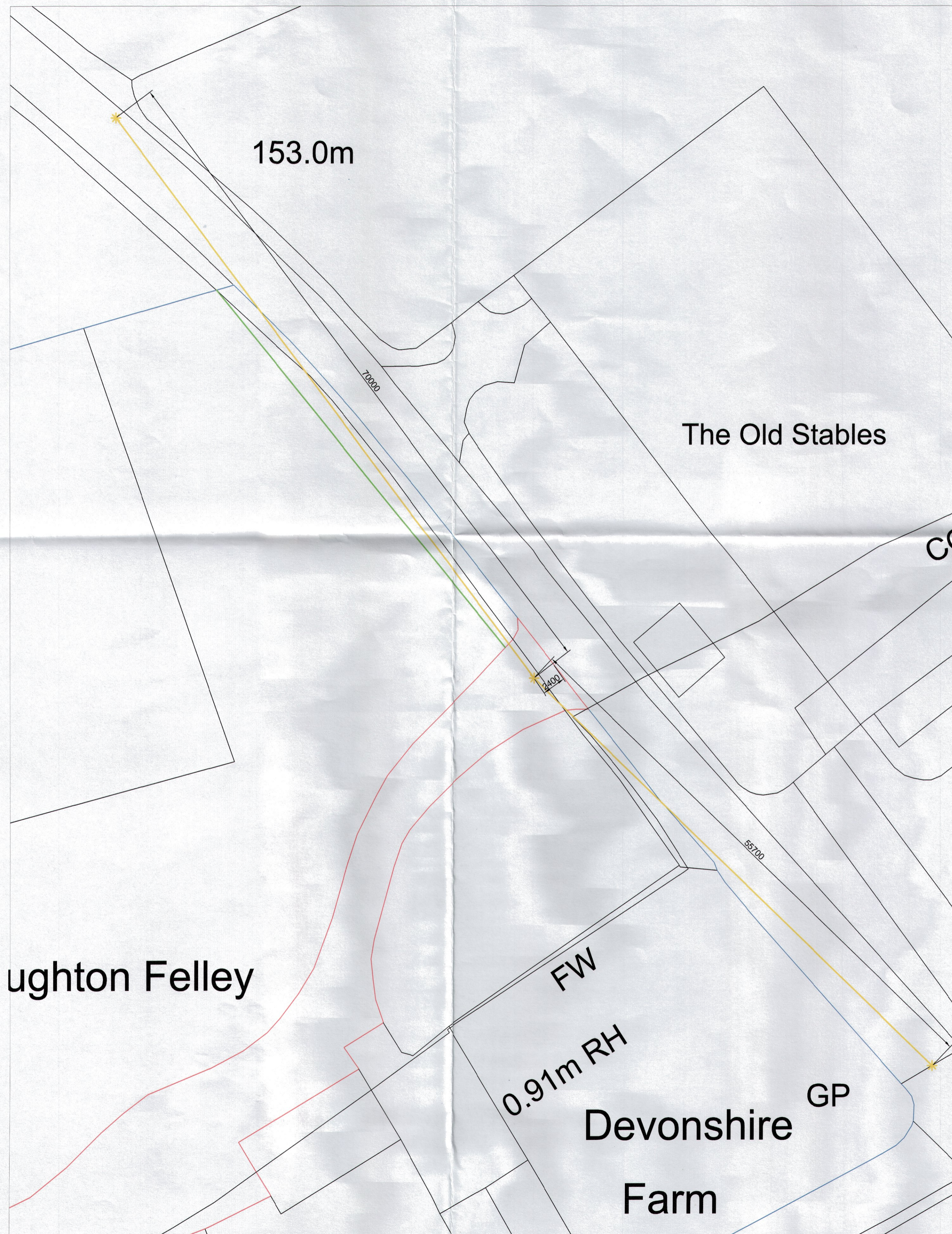
Site Plan Demonstrating Vision Splays To The North & South Of The Vehicular Access 70m North and 55.7m South
