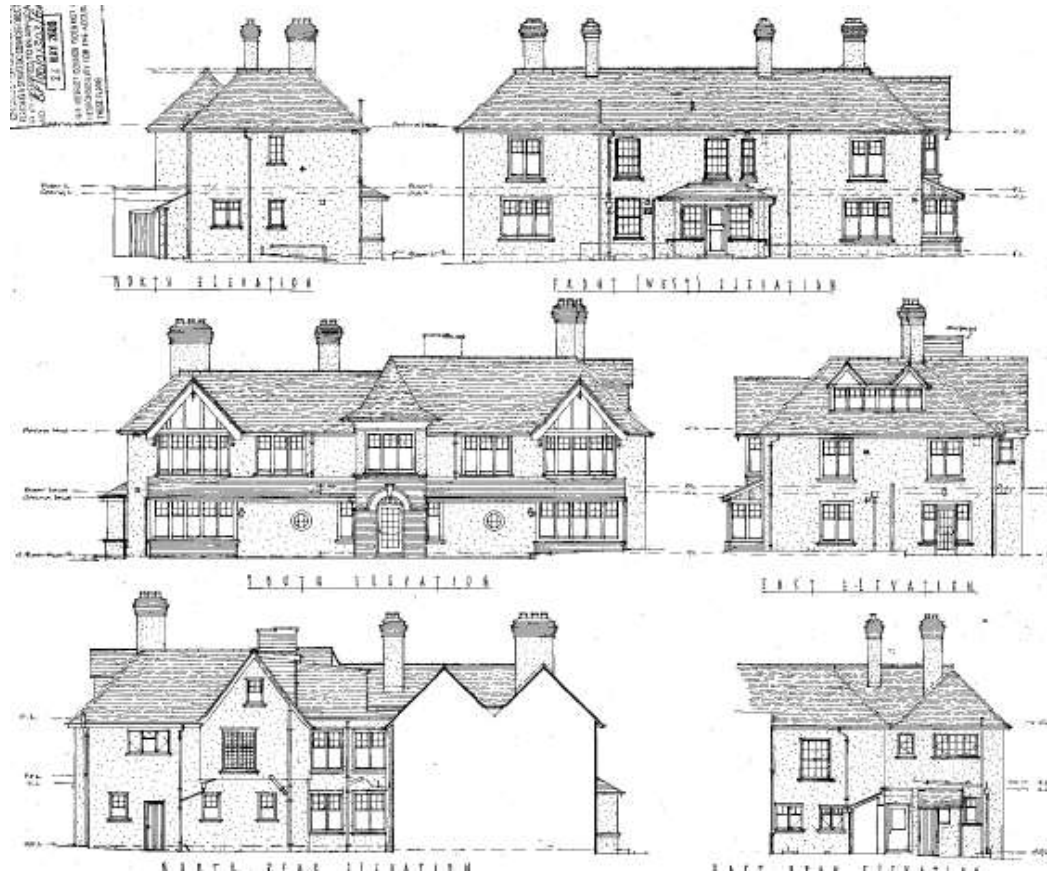
Extract from drawing showing existing elevations in 2000 (not to scale) – of particular note is the variation in the ridge height and the different style of dormer window
